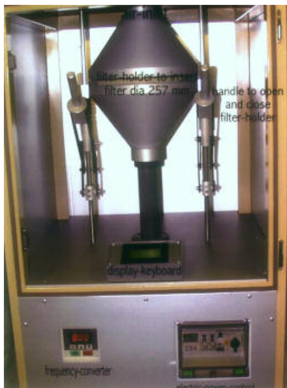
Figure 12: The High-Volume-Sampler (HVS) as used for the pilot monitoring in Damascus.
